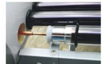
Cover up dust ring carefully
