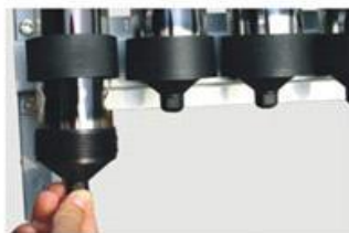
Insert vacuum tubes into tube jacket
